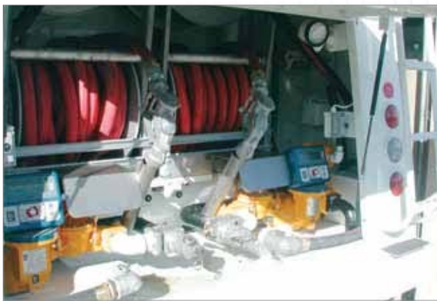
Nozzle Holders that drain directly into rear drain pan – weld on type
