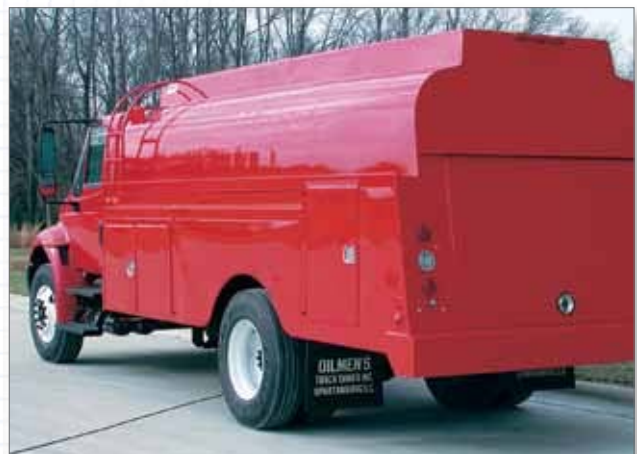
5" Catwalk on Full Skirted Steel Tank
