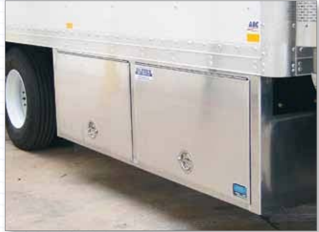
Bolt on Cabinet with Two Fold Up Doors – Used for Long Cabinets
