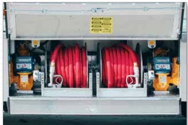
Weld on cabinet with fold up and fold down doors. Used to keep fold up door to smaller size.
