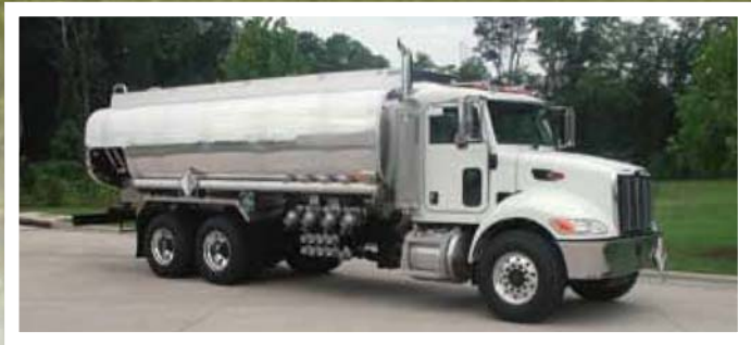
4400 Gal, 4 Compartments, Dual Systems, Bottom Loading
