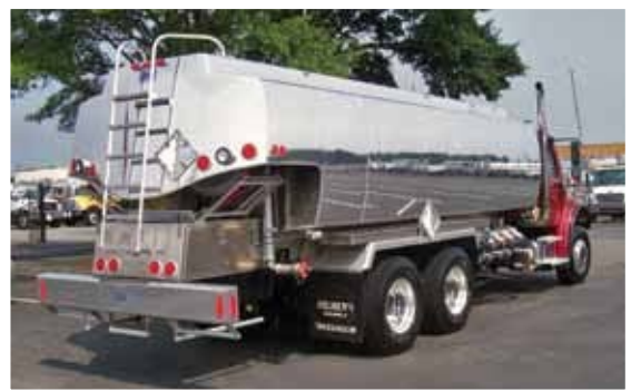
4400 Gal, 4 Compartments, Dual Systems, Bottom Loading
