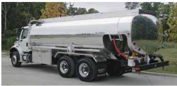
4400 Gal, 4 Compartments, Dual Systems, Bottom Loading
