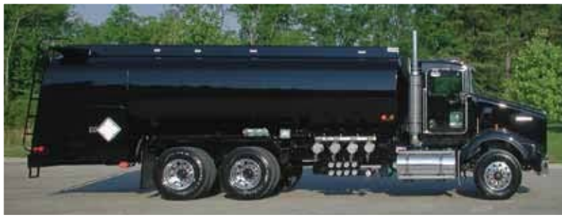
4000 Gal, 4 Compartments, Dual Systems, Bottom Loading
