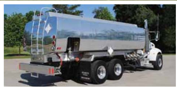
4400 Gal, 4 Compartments, Dual Systems, Bottom Loading
